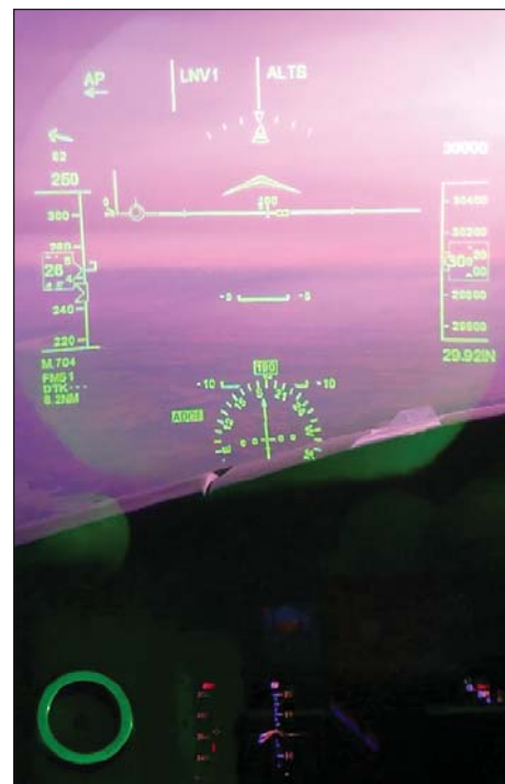
Aftermarket programs for HUD and enhanced flight vision technology are becoming available for a variety of bizjet aircraft. Programs such as Jetcraft's HUD Vision Access include technical and financial analysis incorporating operational and residual value benefit to your aircraft. Shown is the new Kollsman AT-HUD offered in the Jetcraft program during design (above) and in flight (R).
