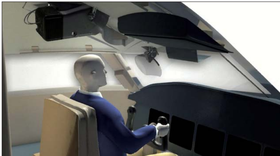
Aftermarket programs for HUD and enhanced flight vision technology are becoming available for a variety of bizjet aircraft. Programs such as Jetcraft's HUD Vision Access include technical and financial analysis incorporating operational and residual value benefit to your aircraft. Shown is the new Kollsman AT-HUD offered in the Jetcraft program during design (above) and in flight (R).
