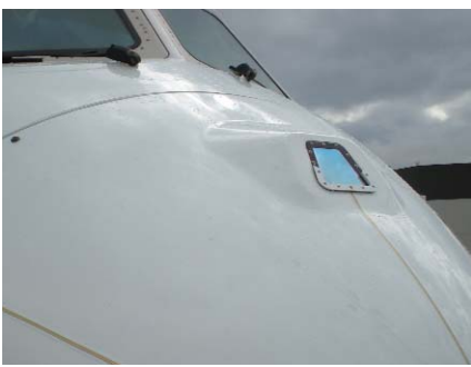
(L-R) Aftermarket installations of Kollsman EVS II sensor in a Boeing 757, McDonnell Douglas MD10 and Bombardier Challenger 604. FAA approved EFVS in 2004 as a means to see the required visual cues at decision height even when the human cannot, enabling the approach to continue to 100 ft, where transition to natural vision is required. FAA plans on more advantages with EFVS including taxi and takeoff, and landing in very low visibility.
