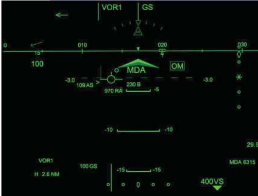
(L) Flight guidance symbology developed for Jetcraft's HUD Vision Access program by Kollsman. (Above) Installation of aftermarket HUDs requires compatible designs for each aircraft installation, as shown in this CAD drawing. (R) Aftermarket developments that include a HUD and EFVS sensor require development, flight test and certification. Here Test Pilot & Designated Engineering Representative Dave Gollings checks out the Kollsman AT-HUD in flight aboard a Challenger 604.
