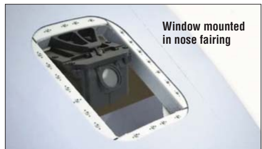
EFVS installations typically include a weather-penetrating sensor, infrared window and processor. Shown here is the Kollsman EVS II.
